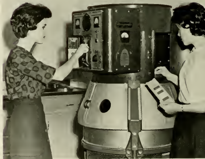
Home Economics Students test fading scientifically with a clothing fadometer.
