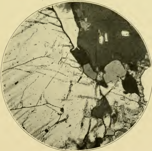
b. Microstructure of hypersthene-akerite showing curved allite lamellae between crossed nicols ( \times 53 ).
