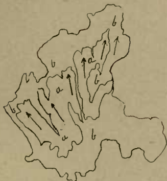
FIG. 38. INTERGROWN ORTHOCLASE (a) AND DEFORMED ORTHOCLASE (b) IN PSEUDOSPHERULITIC OR LAMELLAR STRUCTURE. THE FORMER SHOWS n_g VERY OBLIQUE, THE LATTER n_{111} .
