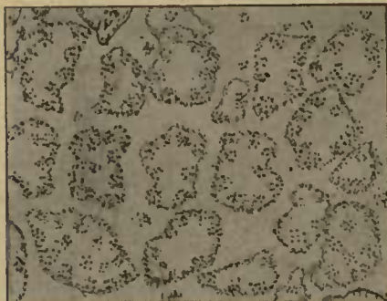
FIG. 20. DISTRIBUTION OF CLUSTERS OF MAGNETITE GRAINS IN THE PERIPHERIES OF SILICEOUS BALLS.
