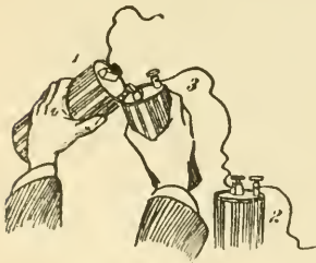
Fig. 181—Touching the carbon to the zinc
