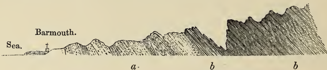
a. Grits and schists; Cambrian (Upper Longmynd) rocks. b. Lingula -schists, with imperfect transverse slaty cleavage (white lines).
