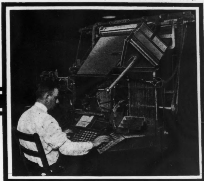
Standardized three-magazine Intertype with three-magazine Power Keyboard Side Unit.
