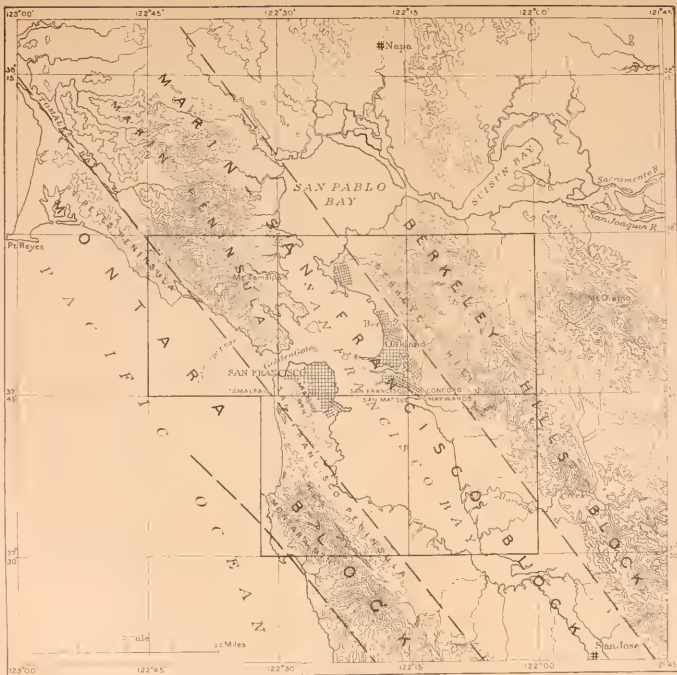
FIGURE 2.—Map of vicinity of San Francisco Bay, showing topographic features and the geomorphic divisions resulting from the adjustment by tilting of great fault blocks.
