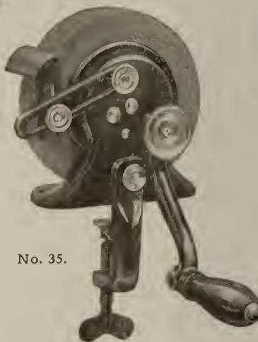
"Compacto"—quickly taken apart or assembled for tool chest service.
