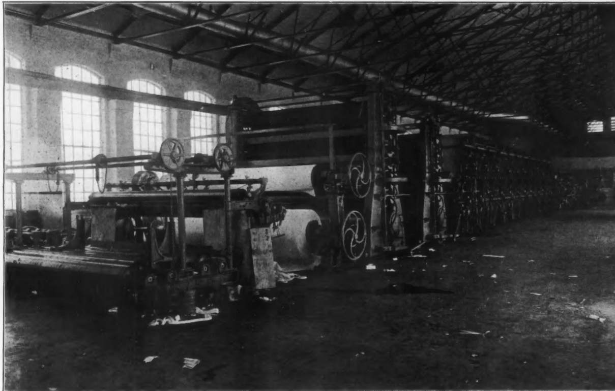
VIEW IN MILL NO. 3 OF THE KALAMAZOO PAPER CO. SHOWING 146" FOURDRINIER
