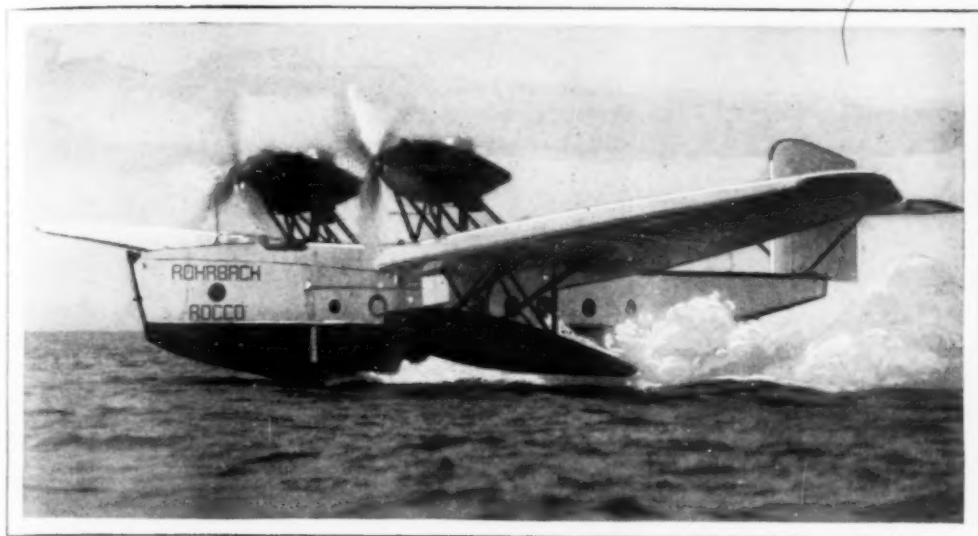
For Faster Trips between Hamburg and London, the Ten-Passenger Flying Boat in Action; Its Two Motors Afford a Speed of 150 Miles an Hour
