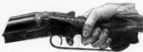
With All the Fingers inside the Trigger Guard, the Gunner Is Less Likely to Suffer Injuries
