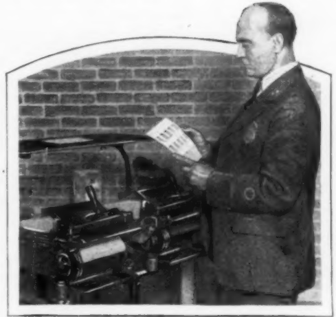
Taking Extra Copies of Fingerprint Records for Police Files; the Duplicating Apparatus in Use
