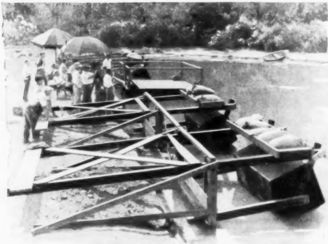
By Rocking These Boxes on Pivots, Realistic Waves Were Produced for a Motion-Picture Scene on Location near Los Angeles
