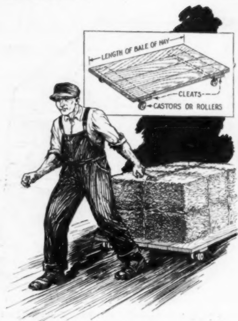
Handy Dolly, Which Can Be Swung in Any Direction, Made from Old Roller Skates
