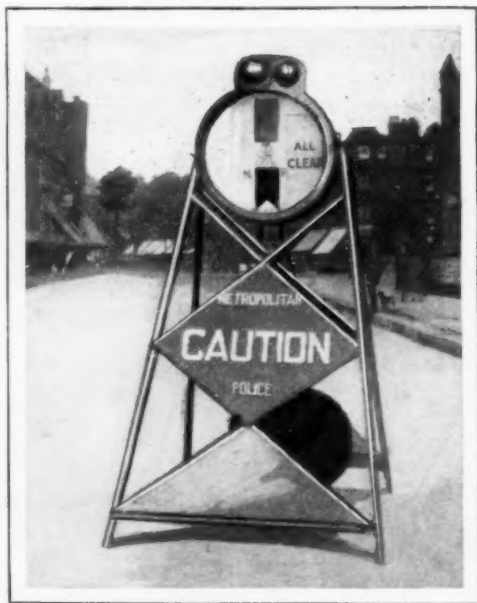
For Traffic Regulation in Curved Street; the Center Guide Tells if There's Anything around Corner
