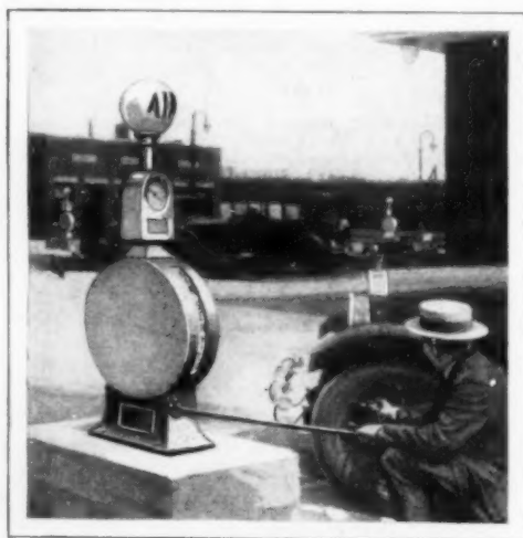
Filling Tire from the Automatic Air Station, Which Shuts Off Supply When Proper Pressure Is Reached
