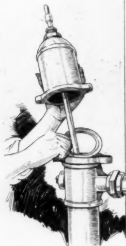
Left, Replacing Air-Dome Gasket; Center, Wiping Off Deck-Leather Seat; Right, Tightening Down Cylinder
