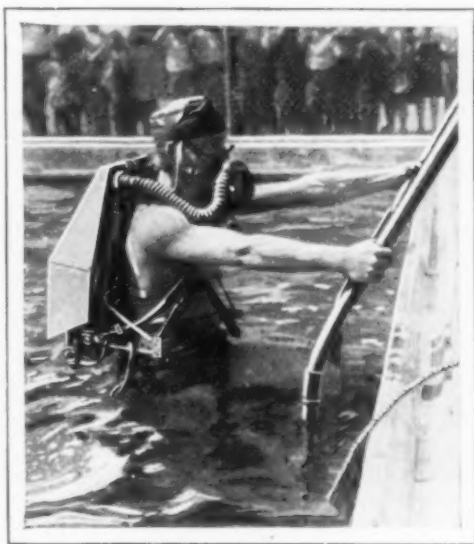
Submerging to Test Fireman's Gas Mask as a Diver's Helmet, Wearer Stayed Under Twenty Minutes
