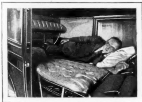
When Not in Use, This Bed for the Auto Tourist Folds Up under the Rear-Seat Cushions
