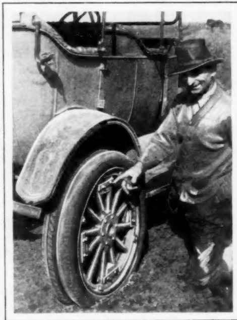
Extra Rear Wheel on Ford Permits It to Cross Freshly Plowed Soft Land
