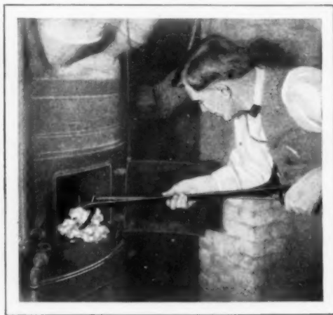
Gripping Tongs That Clutch the Stubborn Clinker, to Effect Its Removal without Shaking the Grates
