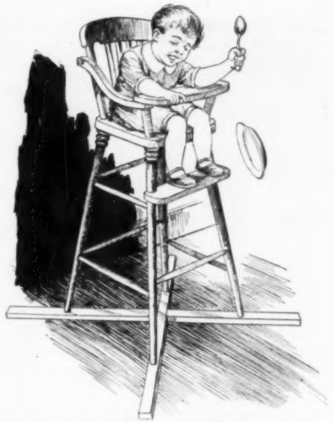
Strips of 1-In. Wood Attached to Baby Chair Prevent It from Tipping
