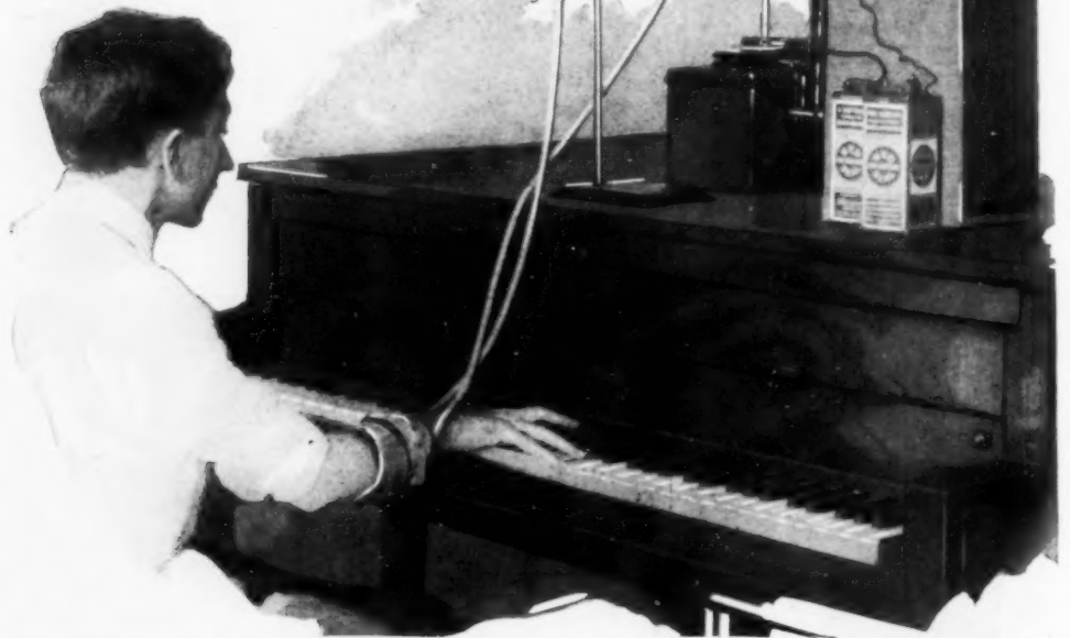
Automatic Recorder to Measure the Muscular Control of a Pianist While He Plays; the Bellows on Each Wrist Actuates the Pair of Pens Which Mark the Revolving Chart
