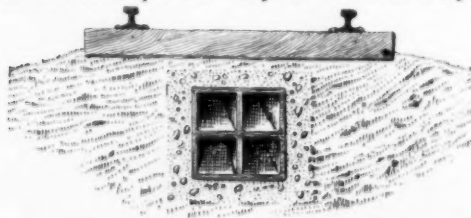
Transmission Ducts Under Tracks
