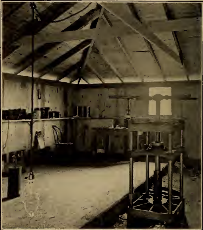
FIG. 1. Interior of Outdoor Laboratory. Shows large press with ice core projecting to right from lateral orifice of iron cylinder. Also shows small press (on table in background) with one of the small cubes between its plates.
