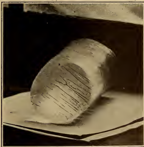
FIG. 4. End view of ice cylinder shown in fig. 3 and photographed at the same time. Shows roughly parallel orientation of crystals, their relative lengths and wedge-shaped terminations.
