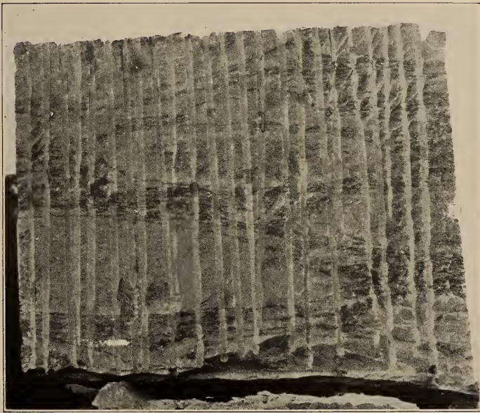
No. 1.—Block of white marble (6 ft. by 4 ft. 6 inches) from the Moretti-Harrah quarry near Sylacauga, Ala., showing lenses bounded by films of muscovite schist. The drilled face is parallel to the strike of bedding.
