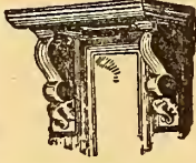
Consoles supporting a cornice.
