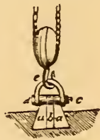
Lewis. a a Dovetail or work of making a lexicon or dictionary. — Section; b Key; c Bolt.
