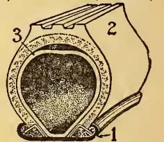
One form of Pneumatic Tire. 1 Rim of Wheel; 2 Casings or Shoe (the Outer "Tube"); 3 Air-Inflated Inner Tube.
