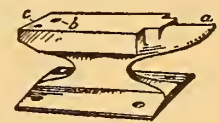
Anvil. a Horn; b , c Holes for Set Chisels, Swage Blocks, etc.
