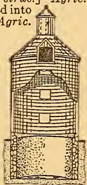
One form of Silo; partly in section.
