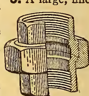
Pipe Union, partly cut away to show construction.
