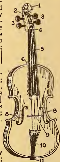
Violin (Stradivarius). 1 Scroll; 2 Peg Box; 3, 3 Pegs; 4 Nut; 5 Finger board; 6 Neck Plate; 8, 8 Sound Holes; 9 Bridge; 10 Tailpiece; 11 Button.
