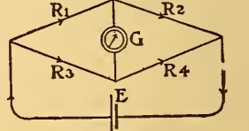
Diagram of Wheatstone's Bridge. R1, R2 Resistances to be compared; R3, R4 Known Resistances, which can be varied; G Galvanometer; E Battery. When G shows no current, R1 : R2 = R3 : R4.
