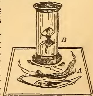
Anamorphoscope. A Dis- torted Picture; B Mirror, showing Normal Image.
