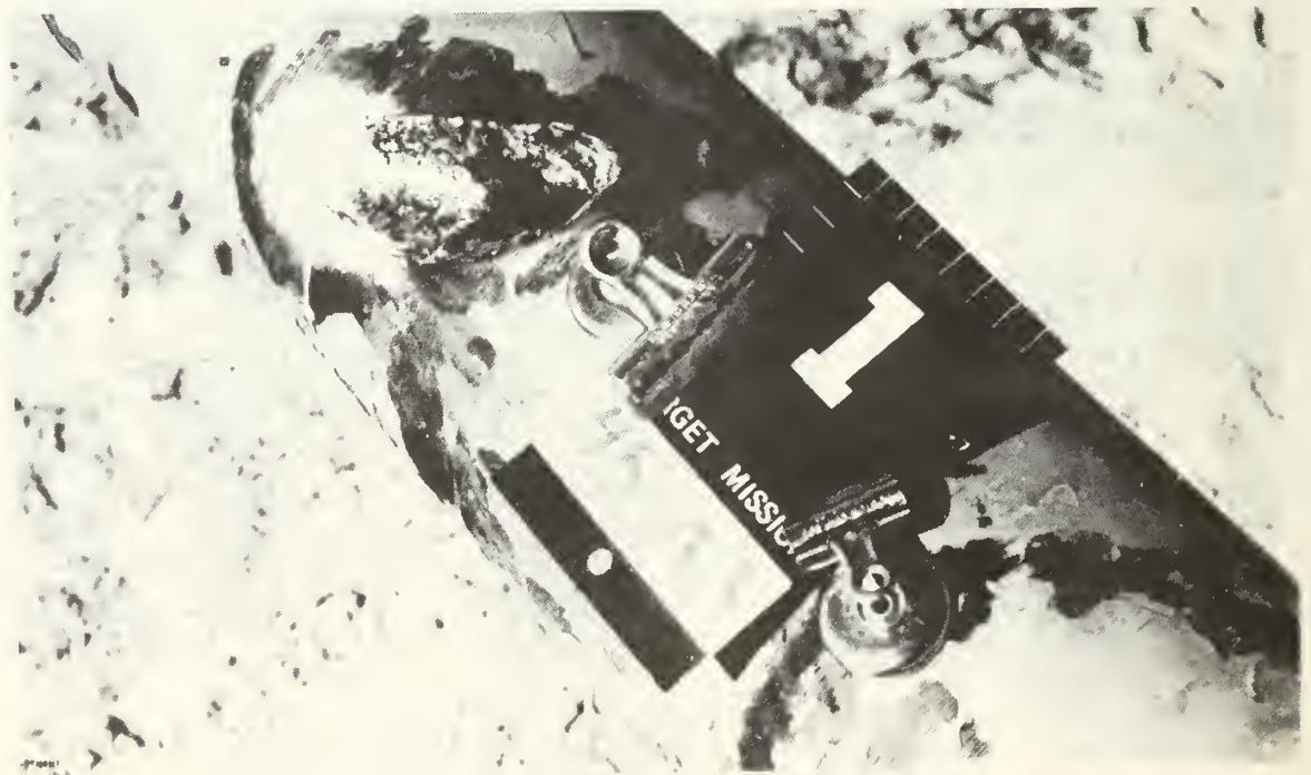
FIGURE 125. Impact One, Target 45, Top of Gun Tube Wall Perforated, Maximum Hole Dimension 37mm.
