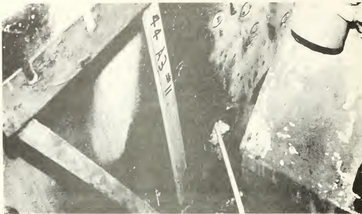
FIGURE 119. Impact Eleven, Target 44, which Perforated the Left Hull Armor into the Engine Compartment.
