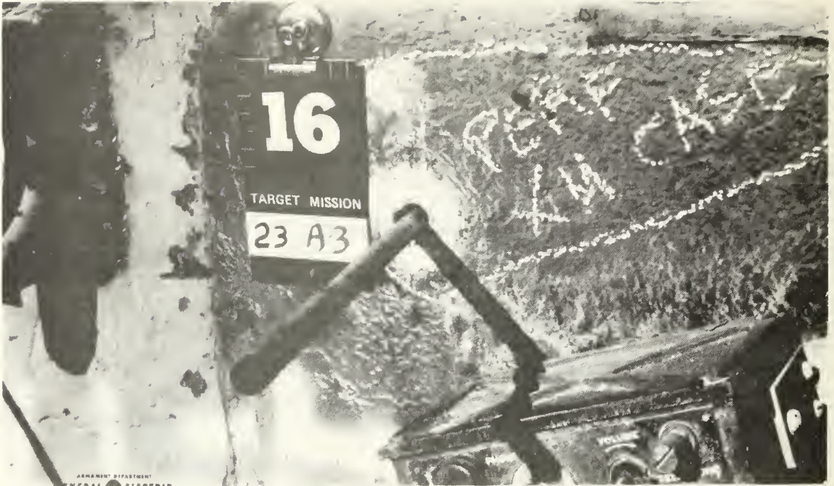
FIGURE 35. Impact Sixteen, Target 23, Perforation of Rear Hull Armor into the Transmission Compartment, Which penetrated the Transmission Thermostat and Cross-Over Line.
