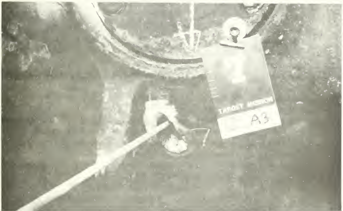
FIGURE 9. Impact Seven, Target 2, Perforation of Rear Hull Armor and Penetration into Transmission Case.
