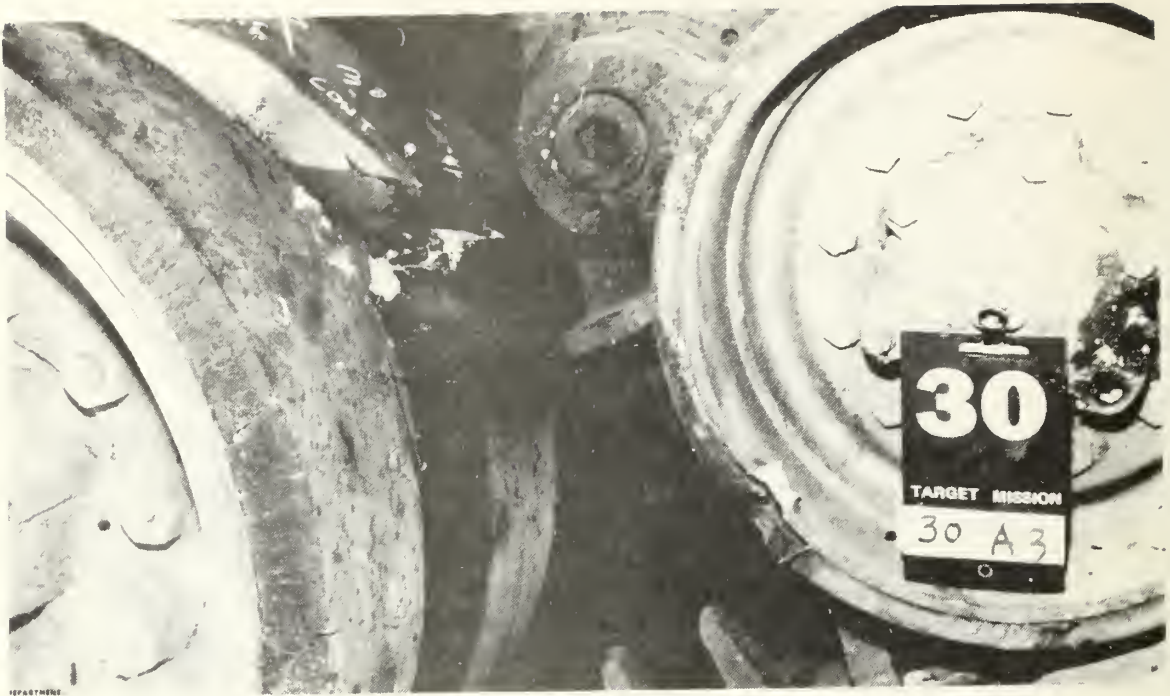
FIGURE 54. Impact Thirty, Target 30, Perforation of Bottom Hull Armor and Penetration into Left Fuel Tank. (Initial Impact was on Left Track Tension Idler Wheel and Left Number 6 Roadwheel)
