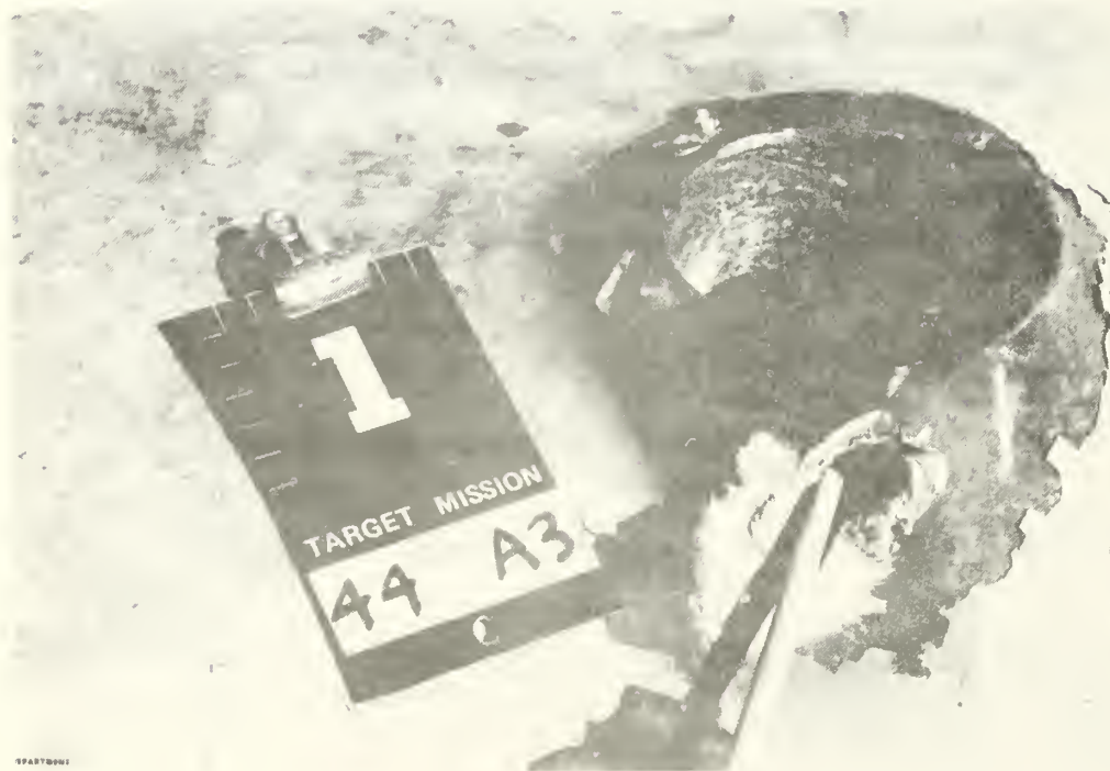
FIGURE 120. Impact One, Target 44, which Perforated the Left Top of the Turret and caused Commander and Gunner Casualties.
