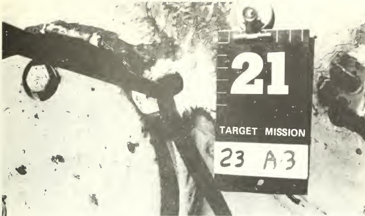
FIGURE 37. Impact Twenty-One, Target 23, Perforation of Rear Hull Armor and Penetration into the Transmission Case.
