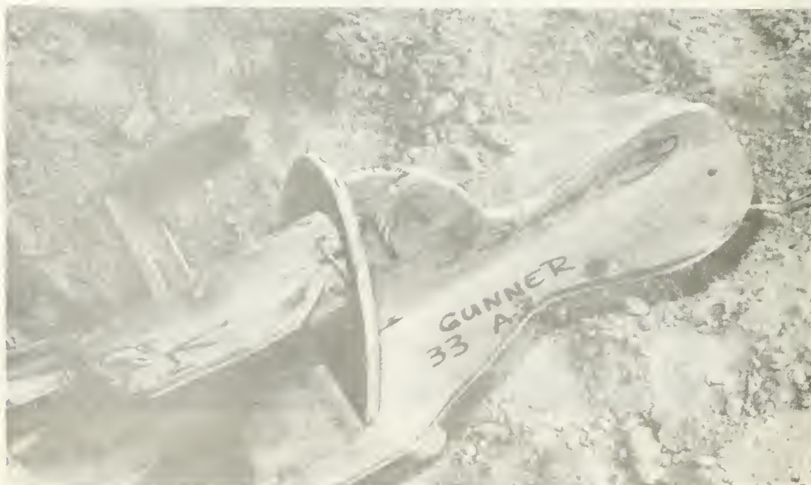
FIGURE 68. Gunner Manikin, Target 33, Showing Damage from Impacts 6 and/or 8, which Perforated the Left Side of the Turret.
