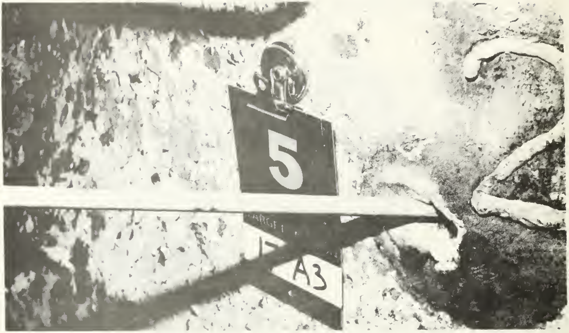
FIGURE 18. Impact Five, Target 17, Perforation of Right Side of Turret.
