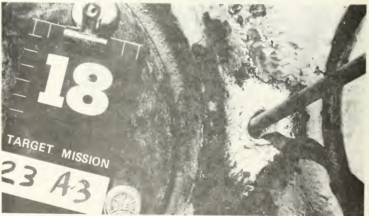
FIGURE 36. Impact Eighteen, Target 23, Perforation of Rear Hull Armor and Penetration into the Transmission Case.
