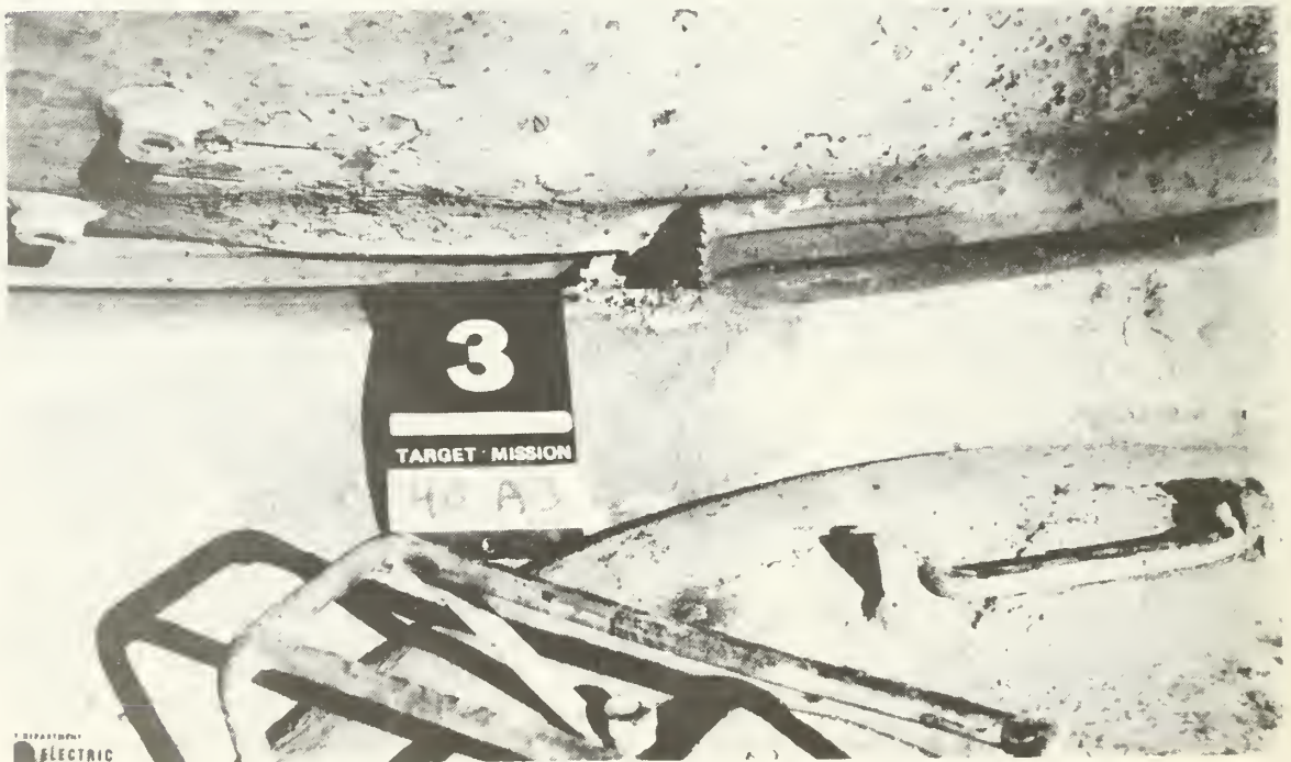
FIGURE 105. Impact Three, Target 40, which Jammed the Turret so that it would not Traverse.
