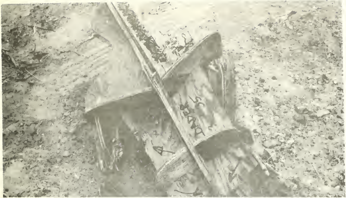
FIGURE 75. Loader Manikin, Target 35, Showing Damage from Perforations into the Fighting Compartment.
