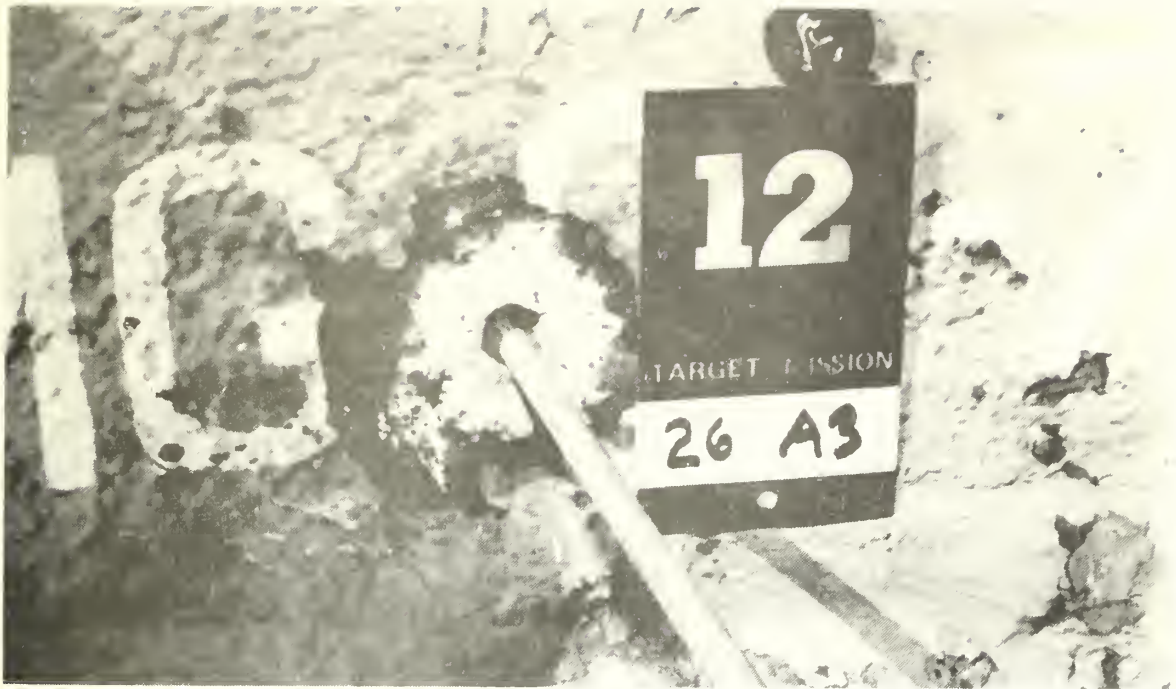
FIGURE 42. Impact Twelve, Target 26, Perforation of Rear Hull Armor and Penetration into the Transmission Case.
