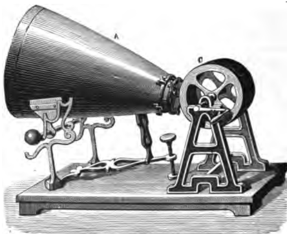
FIG. 5.—Phonautograph of Leon Scott. A, paraboloid resonator, closed at one end by a membrane, to which a light lever is attached. C is a drum covered with smoked paper on which the lever traces a curve. As C rotates it moves from right to left.
