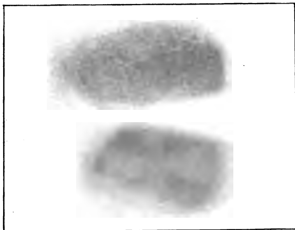
FIG. 1.—REPRODUCTION OF A THIN STRIP OF COPPER, IN FORM OF A CROSS, BY RAYS OF URANIUM ON A PHOTOGRAPHIC PLATE WRAPPED IN BLACK PAPER.
