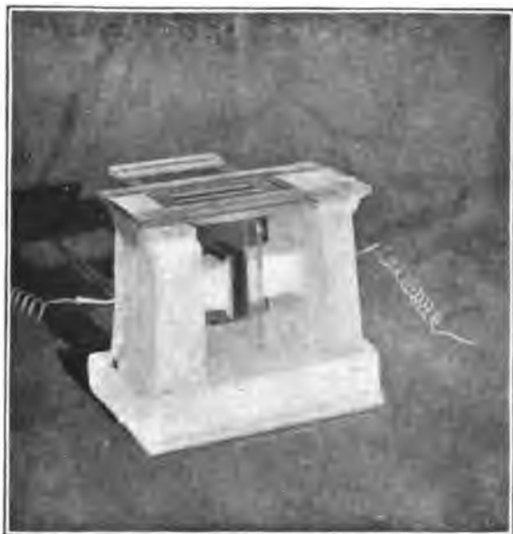
FIG. 10.—APPARATUS FOR PROJECTING ON A PHOTOGRAPHIC PLATE THE SHADOW OF A SCREEN PERPENDICULAR TO THE MAGNETIC FIELD.
