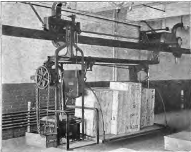
FIG. 2.—TELPER AND TRAILER WITH PLATFORM CARRIER LOADED WITH CASES OF DRY GOODS.
