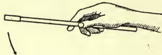
FIG. 21.—SHAKING A DROP OF MERCURY TO THE TOP OF RESERVOIR. (From Biltz.)
