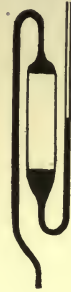
FIG. 19.—INCORRECT FORM FOR RESERVOIR OF BECKMANN THERMOMETER, THE UPPER PORTION OF THE RESERVOIR BEING TOO FLAT.
