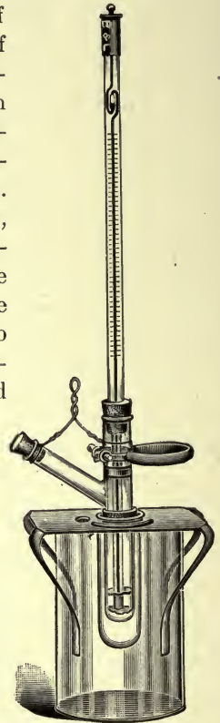
FIG. 22.—IMPROVED MODEL OF BECKMANN FREEZING-POINT APPARATUS WITH MAGNETIC STIRRER.
