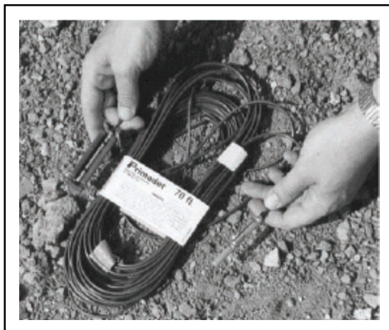
Figure 2-43. M15 Delay Blasting Cap
