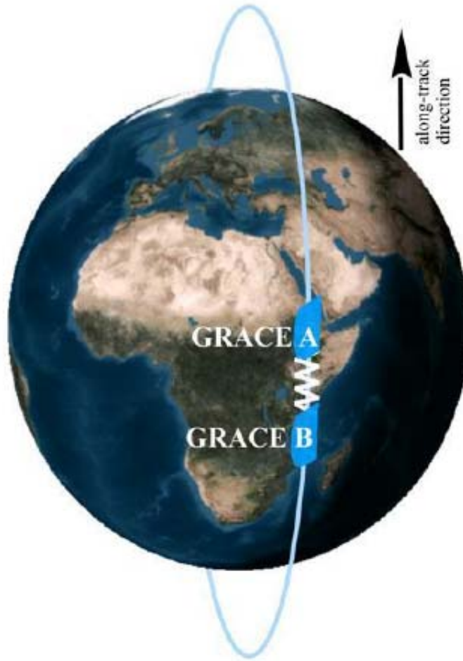
Figure 15. Two satellite inline architecture. Source: [23].
