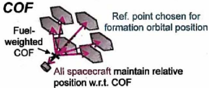
Figure 13. Center of Formation (COF) architecture. Source: [9].
