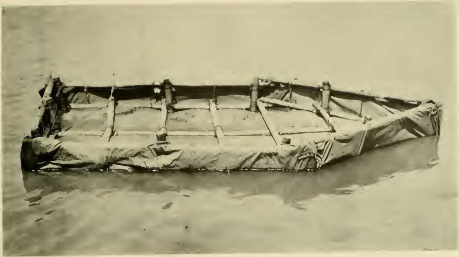
13. BOAT CONSTRUCTED WITH LIGHT SPARS AND A SHELTER-HALF, JONES' POND, CAMP SEVIER, GREENVILLE, S. C.
