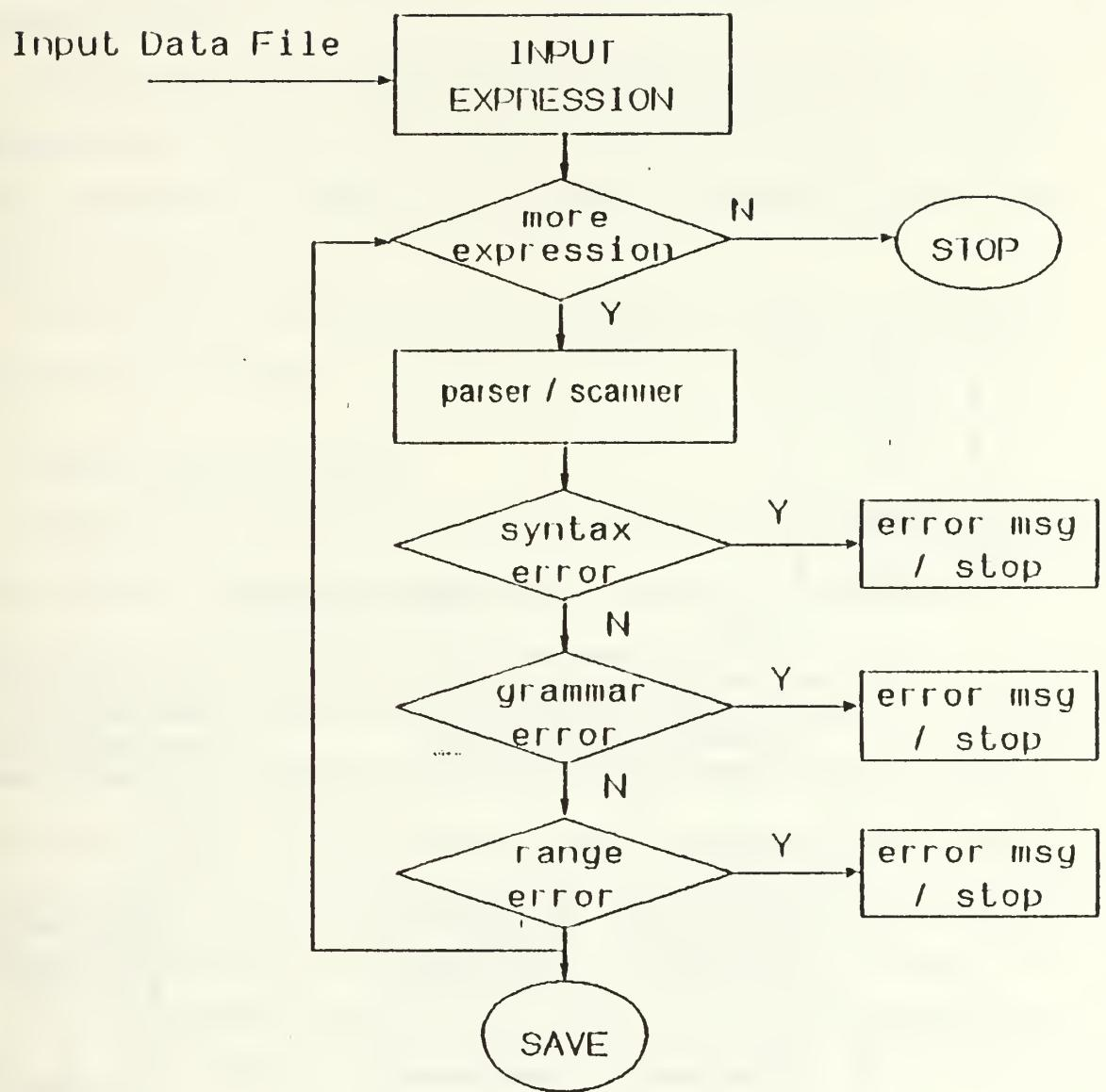
Figure 3.3: Flow Chart of the Data Entry Routine
