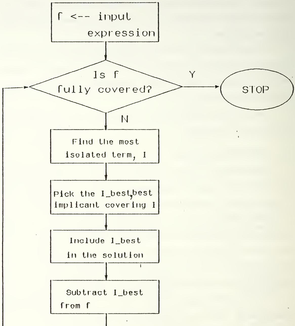
Figure 3.5: Flowchart of Logic Minimization Routine
