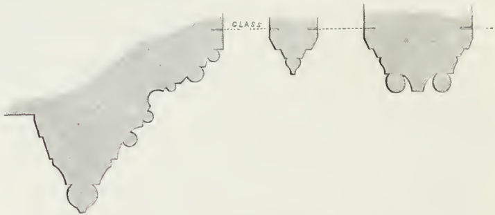
Section of Mouldings.
