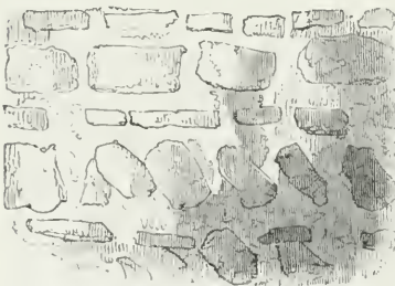
Rubble Masonry, St. Leonard's, Malling, Kent.
