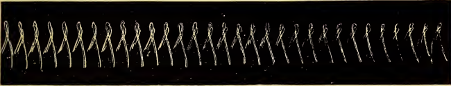
FIG. 79.—Tracings of a Wheatstone rod tuned to the octave, furnished with the wing of a wasp, and arranged so as to register especially the upper loop of the 8.
