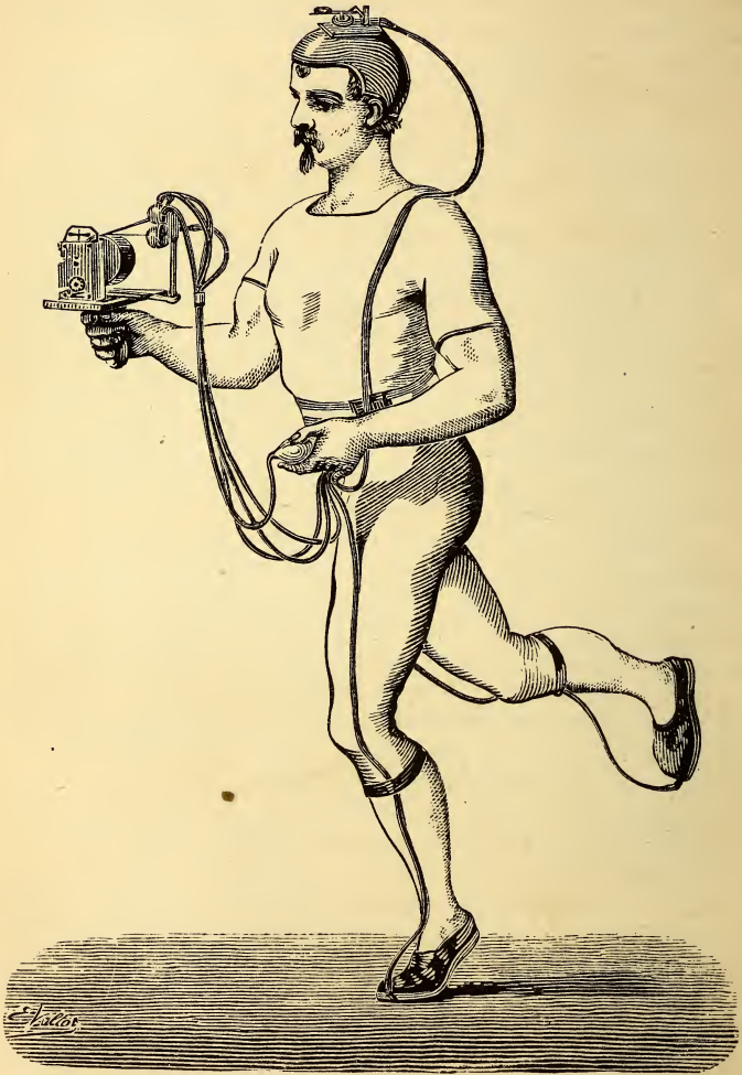
FIG. 27.—Runner provided with the apparatus intended to register his different paces.
