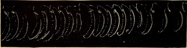
FIG. 77.—Tracing obtained with the wing of a bee, oscillating in a plane which is sensibly tangential to the generatrix of the registering cylinders.
