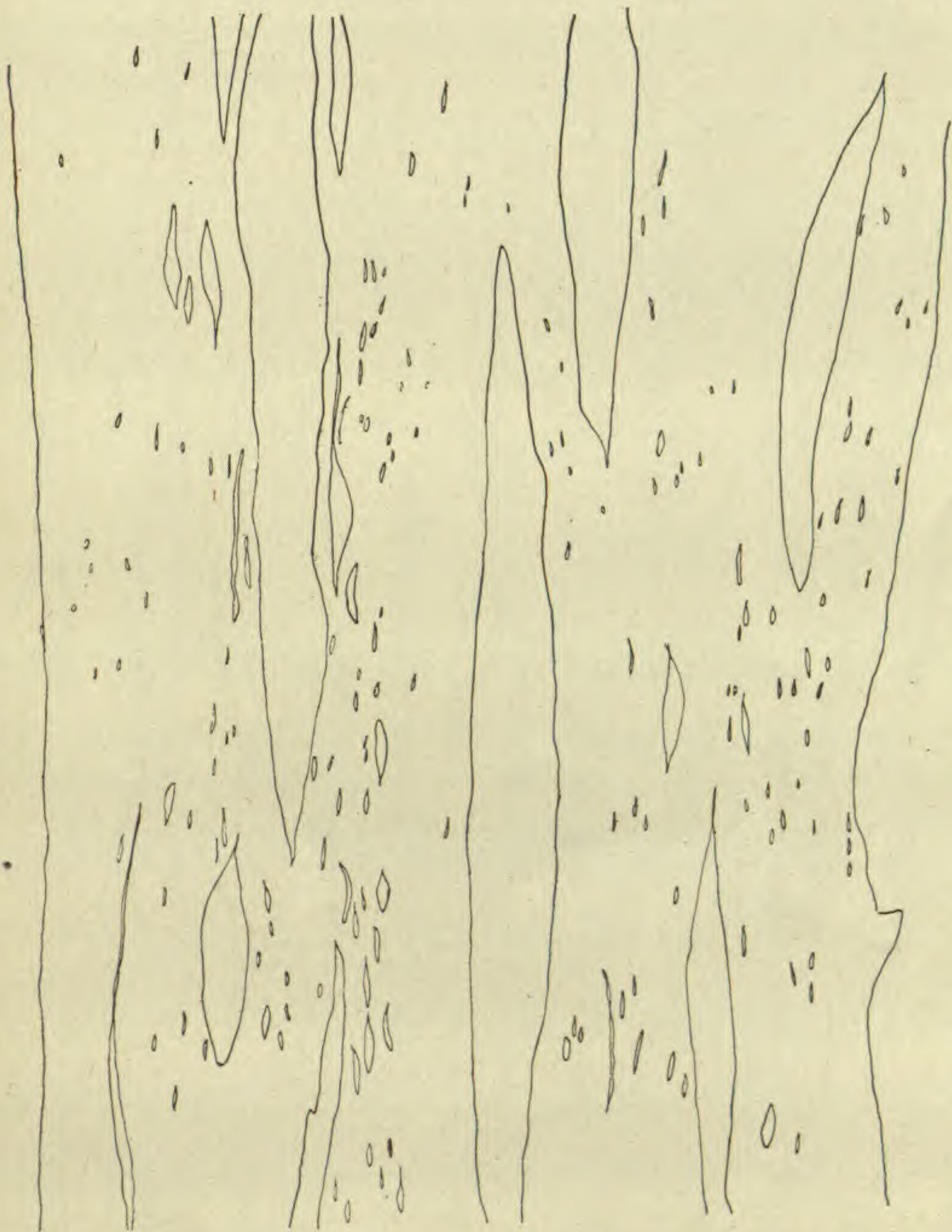
FIG. 2. A 2.5 per cent agar gel after drying at about 43° C. and soaking in water, X 57.
