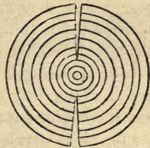
68. Effect of Seasoning of Round Timber, showing the Shrinkage greatest in the outer Wood.
