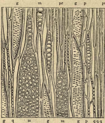
52. Vertical Section of Beech Wood, in a Plane tangent to Rings of Annual Growth.
