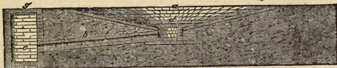
119. Foundation of a Tar-kiln, in which a, d, i : a sloping brick or stone hearth, with a grating at d , through which the tar passes, and is conducted by the pipe, b , to the reservoir, c .
