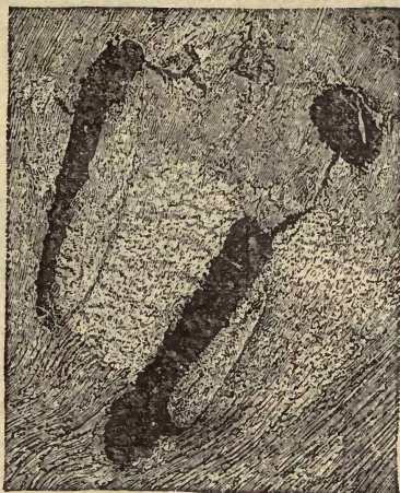
87. Cavities made in Fallen Timber by the Larvæ of Insects, tending to rapidly hasten its Decay.
