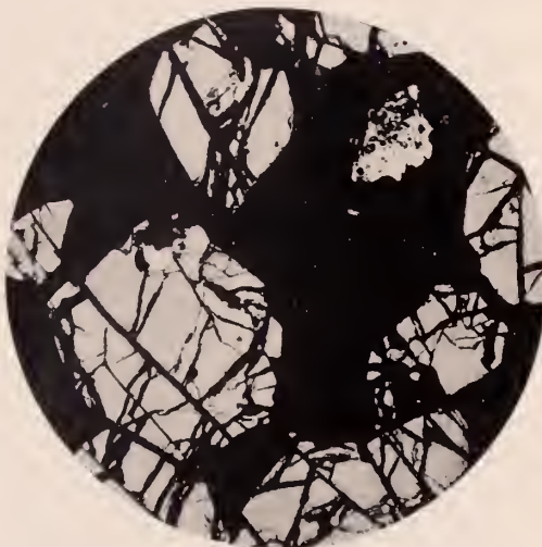
Benrose, Collo., Derby. Fig. 4.— \times 23 . Spandite (manganese-garnet), in psilomelane. Rámabhadrapuram, Vizagapatam district.
