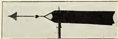
U. S. Weather Bureau A RECORDING WIND VANE
