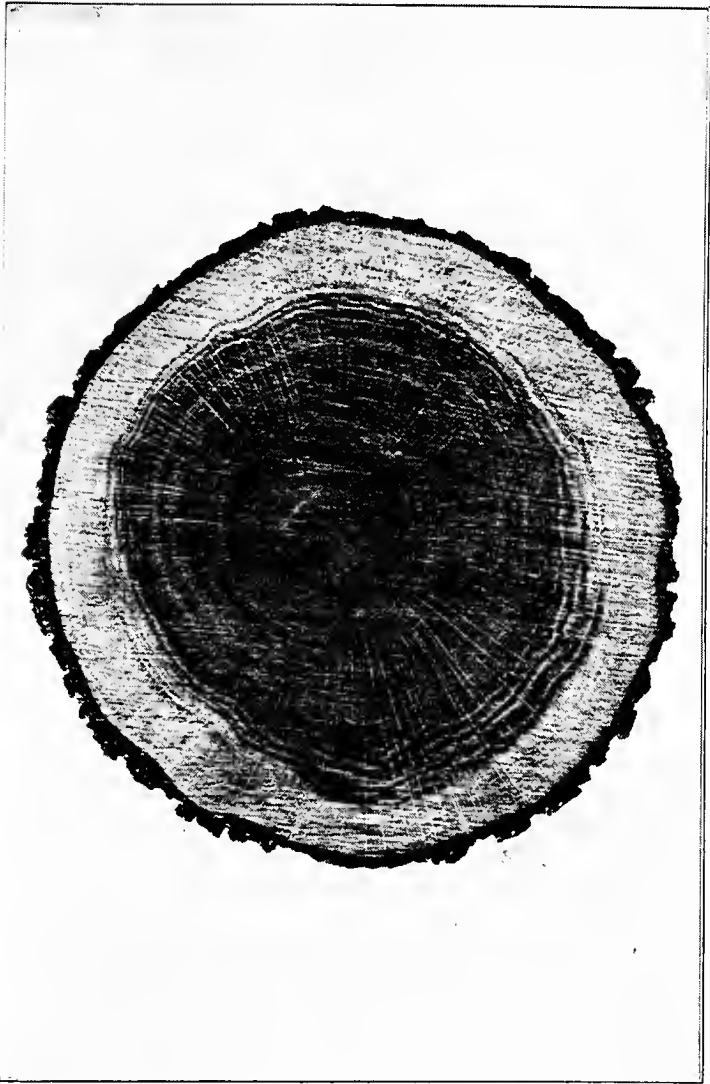
Transverse Section of Trunk of White Oak, Quercus alba , Showing Bark, Sapwood, Heartwood, Annual Rings and Medullary Rays.
