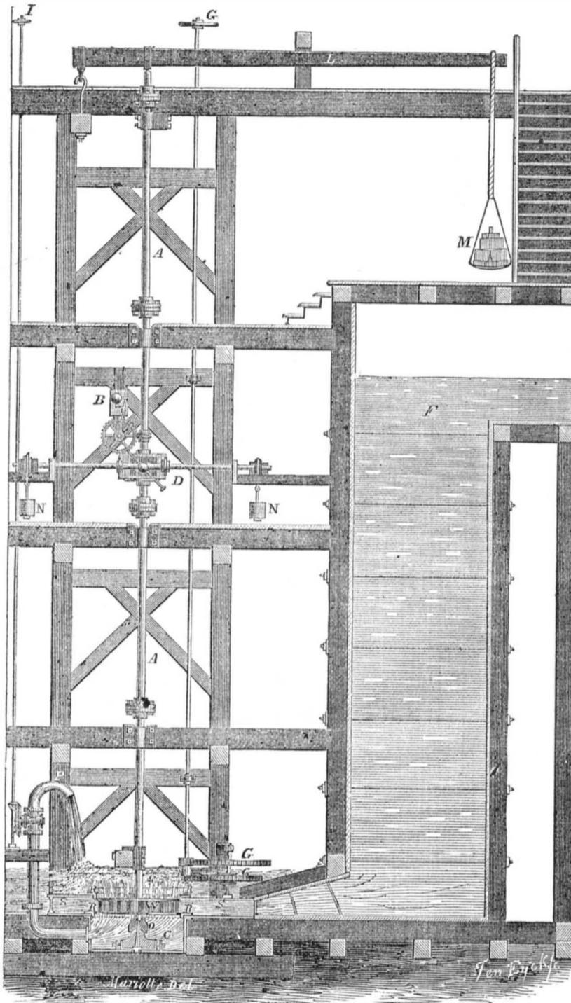
The accompanying figure is an elevation of Reuben Rich's patent Center Vent Wheel with a cast iron scroll, to which is applied Winters' Hydrostatic Chamber. This view represents a wheel in successful operation at the cotton mills of the Tallassee Manufacturing Co., at Tallassee, Ala. A "Prony Brake" for ascertaining the power of the wheel, is also represented.
