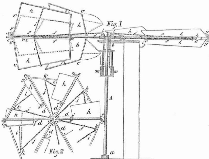
The accompanying engravings represent an improvement in Windmills for which a patent was granted to J. S. Morgan, of Highland, Madison Co., Ill., on the 17th of July last. Fig. 1 is a side elevation of the windmill, and fig. 2 is a top view of it. Similar letters refer to like parts.
