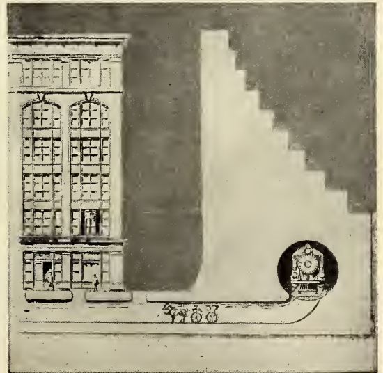
SECTIONAL VIEW OF A LOCK, AS HIGH AS A SIX-STORY BUILDING. THE TUBE THROUGH WHICH THE WATER IS ADMITTED IS LARGE ENOUGH TO HOLD A LOCOMOTIVE.
