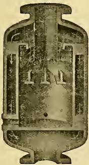
Fig. 23-91. Class B. Vertical. For maximum working pressure of 150 pounds per square inch. Sizes—2 to 12-inch.
