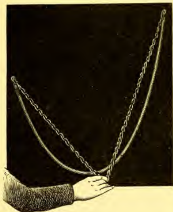
THE CATENARY, OR CURVE FORMED BY A HANGING CHAIN.
