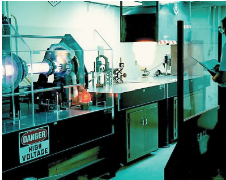
Figure 6. CO 2 Laser Used to Study the Effects of Radiation on Materials[9].
