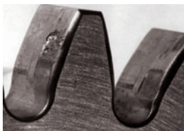
Figure 1. Spalling Failure on the Surface of a Gear Tooth Caused by Surface Fatigue[2].
