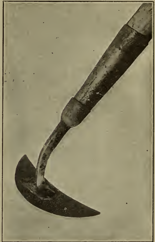
FIG. 4.—A "scuffle" hoe similar in principle to that shown in figure 3, devised by A. B. Leckenby, Seattle, Wash. The blade of either of these hoes may be made from an old saw blade.
