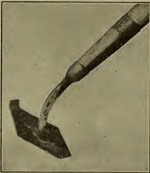
FIG. 3.—A "scuffle" hoe devised and used by W. J. Langdon, Sumner, Wash., in thinning and weeding root crops. A very effective implement.
