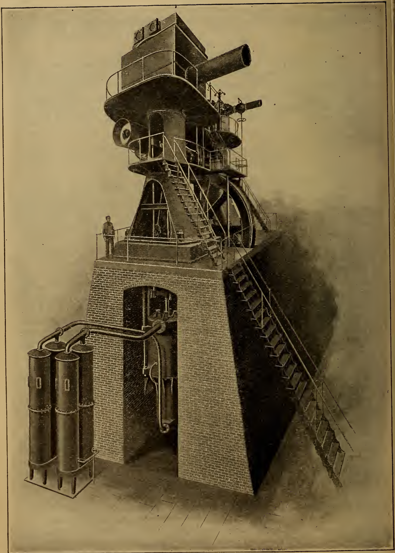
FIG. 151—THE VERTICAL FOUR STAGE HIGH PRESSURE AIR COMPRESSOR USED FOR SUPPLYING POWER FOR STREET CAR SERVICE ON THE 28TH AND 29TH STREET LINES, NEW YORK.
