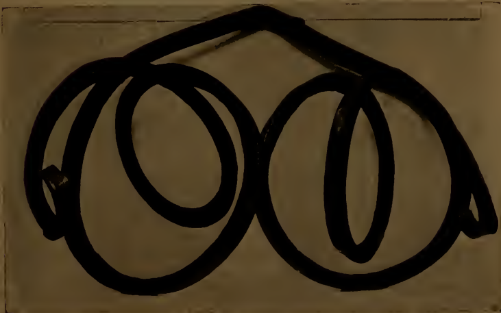
FIG. 484—CHIP OF STEEL TAKEN OFF BY A BOYER PNEUMATIC HAMMER.
