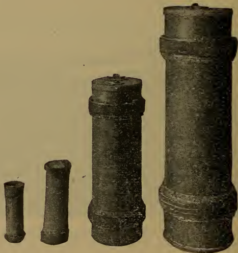
Fig. 342.—(1) Carrier used in the Berlin system; (2) Largest carrier used in the London system; (3) Six-inch carrier used in the first Philadelphia system; (4) Eight-inch carrier used in New York and Boston.
