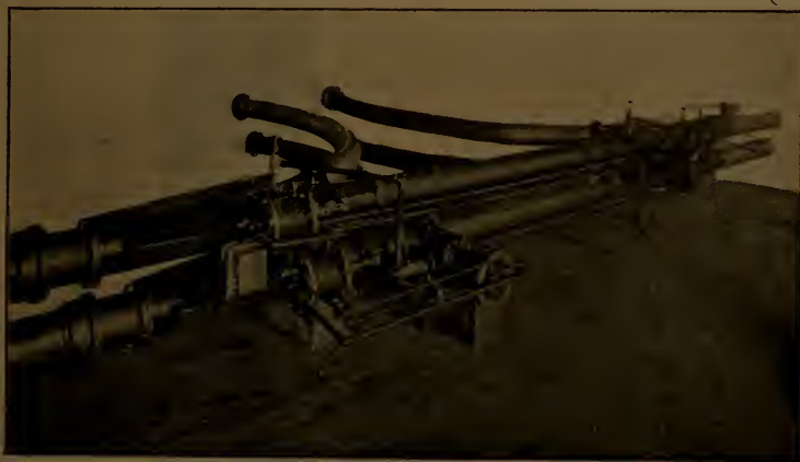
FIG. 341.—SET OF CUT-OFF SWITCHES FOR EIGHT-INCH PNEUMATIC TUBES.
