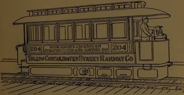
FIG. 146—THE MEKARSKI SYSTEM AT TOLEDO, OHIO.
