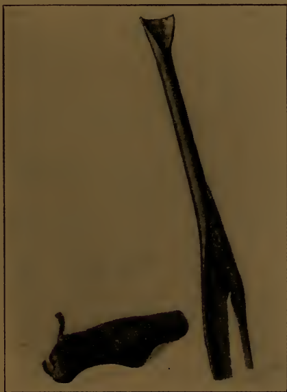
FIG. 278.—TUBES EXPLODED BY MEANS OF COTTON WASTE SATURATED BY LIQUID AIR.
