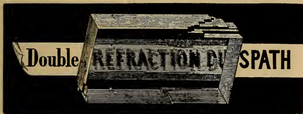
Fig. 17.—Double refraction of Iceland spar.
