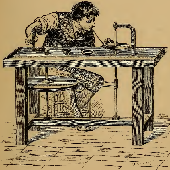
Fig. 125.—Apparatus for Sawing Hard Stones.
