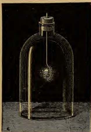
Fig. 33.—Combustion of the Diamond in Oxygen.
