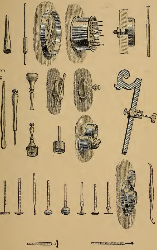
Fig. 124.—Tools and other objects used by the Engravers of Hard Stones.
