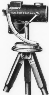
Fig. 1.—A Portable Illumination Photometer.
