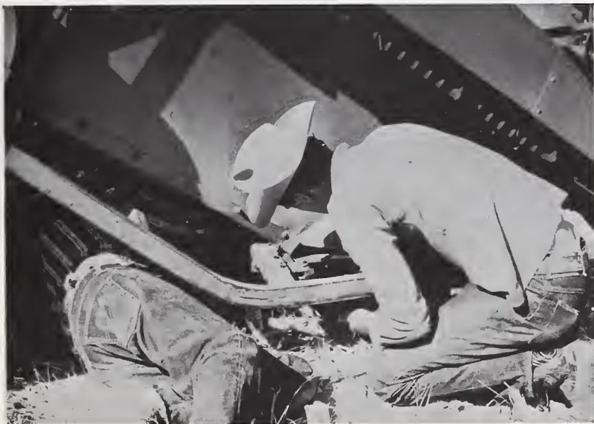
As part of the Extension management training course, two employees of the Ute Tribal Livestock Enterprise learn how to repair and adjust the knives and feeder chains on a corn chopper to reduce "down time" in the field.
