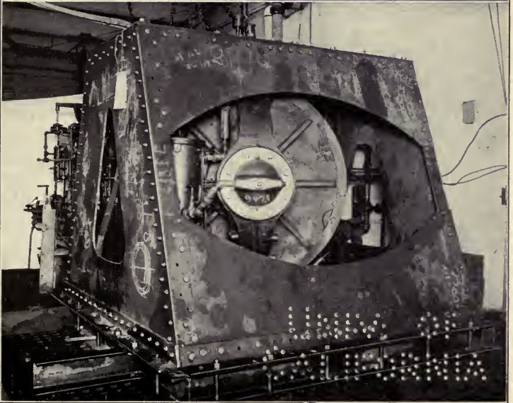
TWO VIEWS OF THE SPERRY SHIP-STABILIZING GYROSCOPE The upper figure shows the precession engine in the foreground
