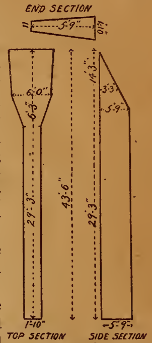
Figure 24. A Straight Vat Known as the Australian Sheep Dipping Tank.
