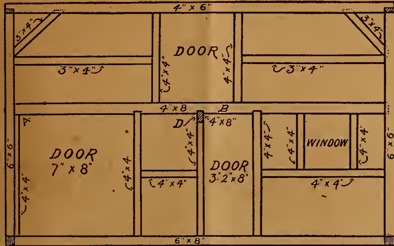
Figure 24. Construction of Ends of $425.00 Barn.
