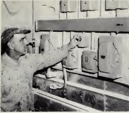
Through these controls a farmer dries 144 bushels of shelled corn and small grains in 2 hours, at 30% moisture.
