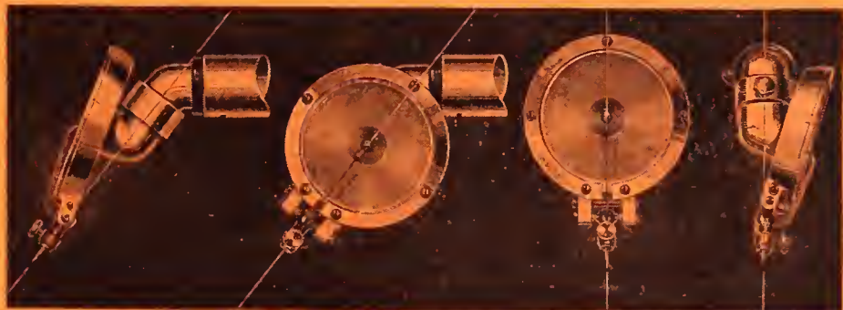
The Reproducer turns on its axis—the needle remaining on exactly the same center and at the same correct angle in both positions
