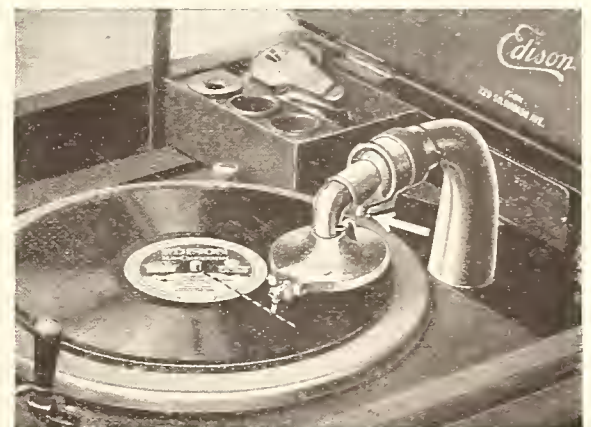
SHOWING POSITION FOR PLAYING EDISON OR OTHER HILL AND DALE CUT RECORDS
