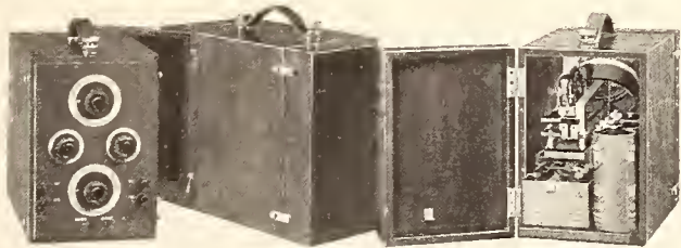
Cutting and Washington Receiver 12A—"Town and Country" model (portable type). A two-tube set which makes an ideal receiver both for the home and for outing use. For either single circuit or double circuit.
