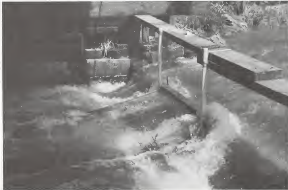
Figure 4.11 – Net-sampler with large wooden frame for coarse bedload at Squaw Creek: a) sampler with 0.30 m by 1.55 m opening and 10 mm mesh width, b) net-sampler in the stream causes only minor flow disturbance.
