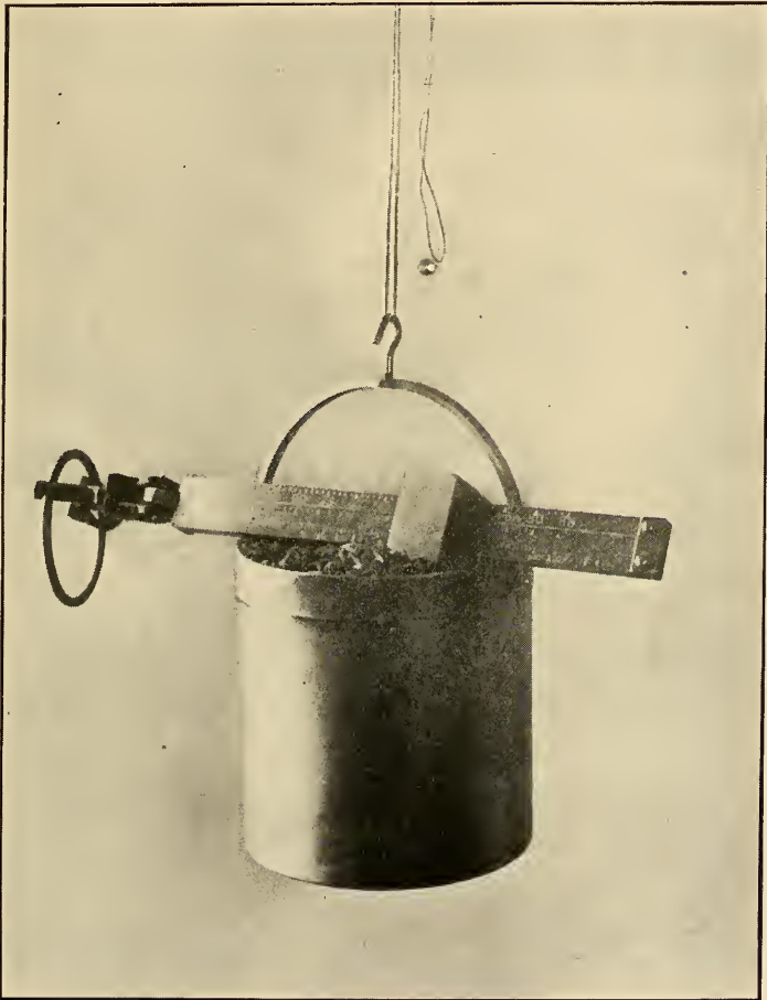
FIG. 43. Standard grain tester. Note the three scales of divisions on the beam.
