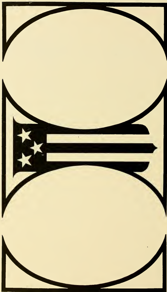
Figure B. Zinc etching made from a pen drawing for printing Senior panel mounts. The zinc etching is made to accommodate oval picture size 3\frac{1}{4} \times 4\frac{1}{2} inches and is made in correct proportion to reduce to 4\frac{3}{4} \times 2\frac{7}{8} inches, which is the desired size of engraving as shown by Figure A.
