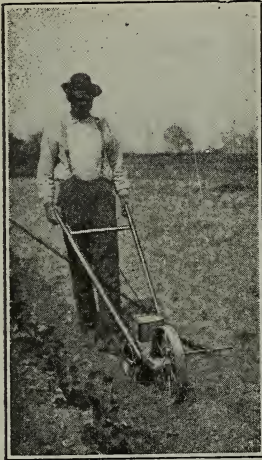
Planet Jr. No. 25, Hill & Drill Seeder at work planting and marking next row.
