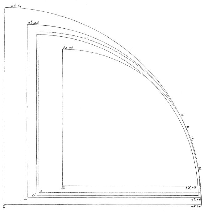
those semi-axes. In the same way ellipses II. and III., as determined above, are drawn. (The parts of these three ellipses between A and D are not drawn in the diagram. The differences in the lengths of the semi-axes are made about eighty times out of proportion, that the differences between the ellipses may be visible.) The dotted ellipse about the centre O is an ellipse equal to the mean ellipse, and so drawn as to
