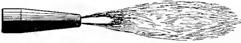
FIG. 23.—More Oxygen Pressure Applied. Flame Contains Slight Excess of Acetylene, and is Known as “Carbonizing.”
