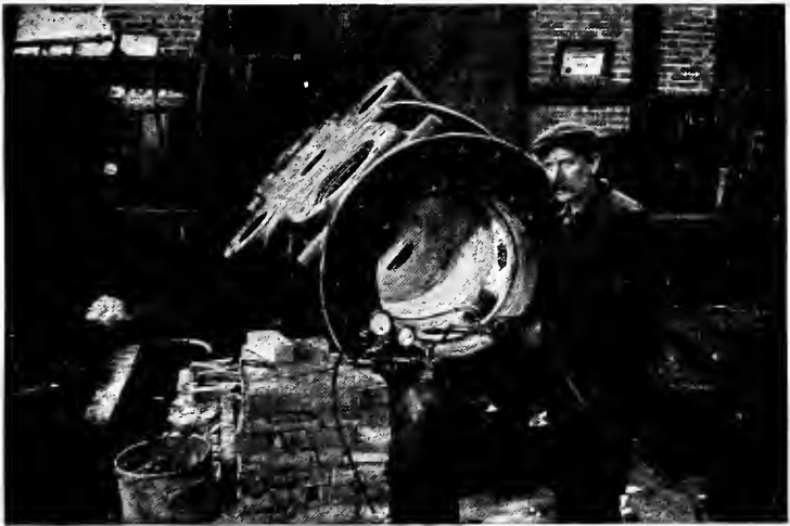
FIG. 52.—View of Locomotive Cylinder with Three Jackets 3 Inches Thick. This job weighed over 16 Tons and Required Fifty-six Hours of Welding.
