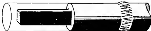
FIG. 67.—Broken Part of Shaft Removed and New Piece Added, thereby Moving the Weld away from the Weak Part.
