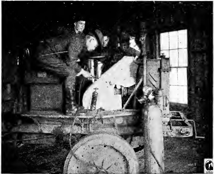
FIG. 86.—Removing Carbon from U. S. Army Truck, by the Oxygen Process, at the Ordnance Welding School.
