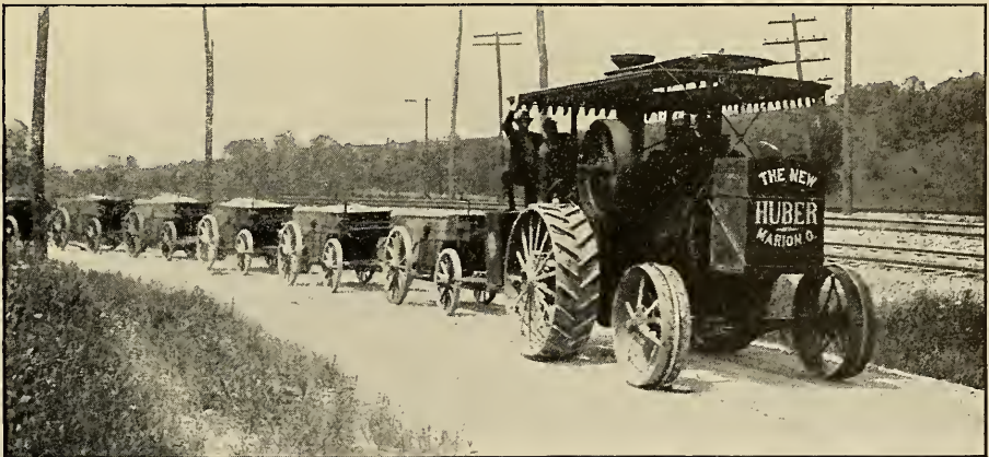
One of the Smaller Sizes of New Huber Traction Engines, Hauling a Train of Wagons Loaded with Crushed Stone.
