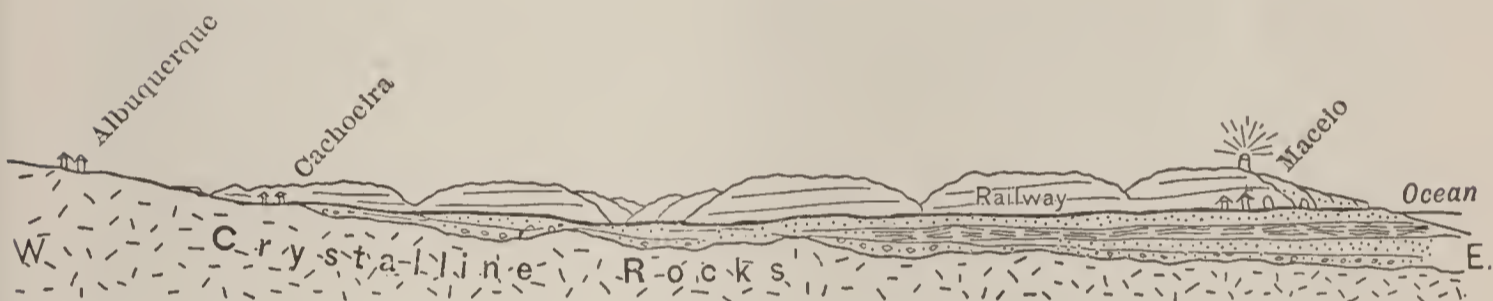
Ideal Section from Maceio to Albuquerque along the Alagôas Railway (35 kilom.), Showing the Eocene Sediments Overlying the Crystalline Rocks.
