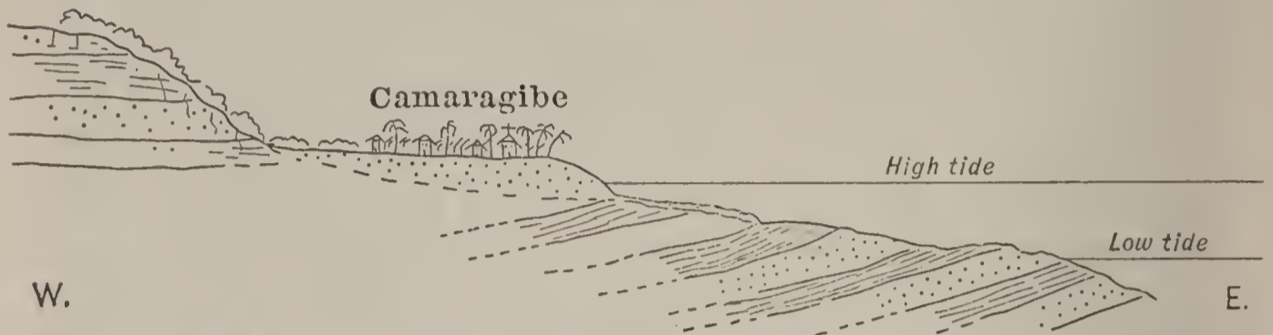
Section through Passo de Camaragibe, Showing the Shales Exposed Between Tides, and their Relation to the Mottled Beds in the Hills back of the Town.
